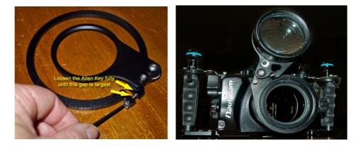
Push the Adaptor onto the housing lens port, so it sits flush to the front of the port. Tighten the Adaptor allen-key screw until the screw begins getting tight, turn slightly further until the Swing Away Mount feels that is firmly attached, but not so tight that it damages the port surround! Make sure the gap in the side of the unit (see below) is getting smaller, but NEVER so tight that the two edges meet. There will always be a small air gap (3 to 5 mm).
